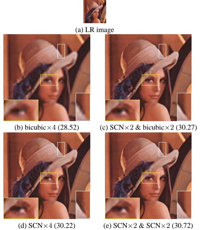
Figure 3. SR results for the “Lena” image upscaled by 4 times. (a) \rightarrow (b) \rightarrow (d) represents the processing flow with a single SCN \times 4 model. (a) \rightarrow (c) \rightarrow (e) represents the processing flow with two cascaded SCN \times 2 models. PSNR is given in parentheses.
