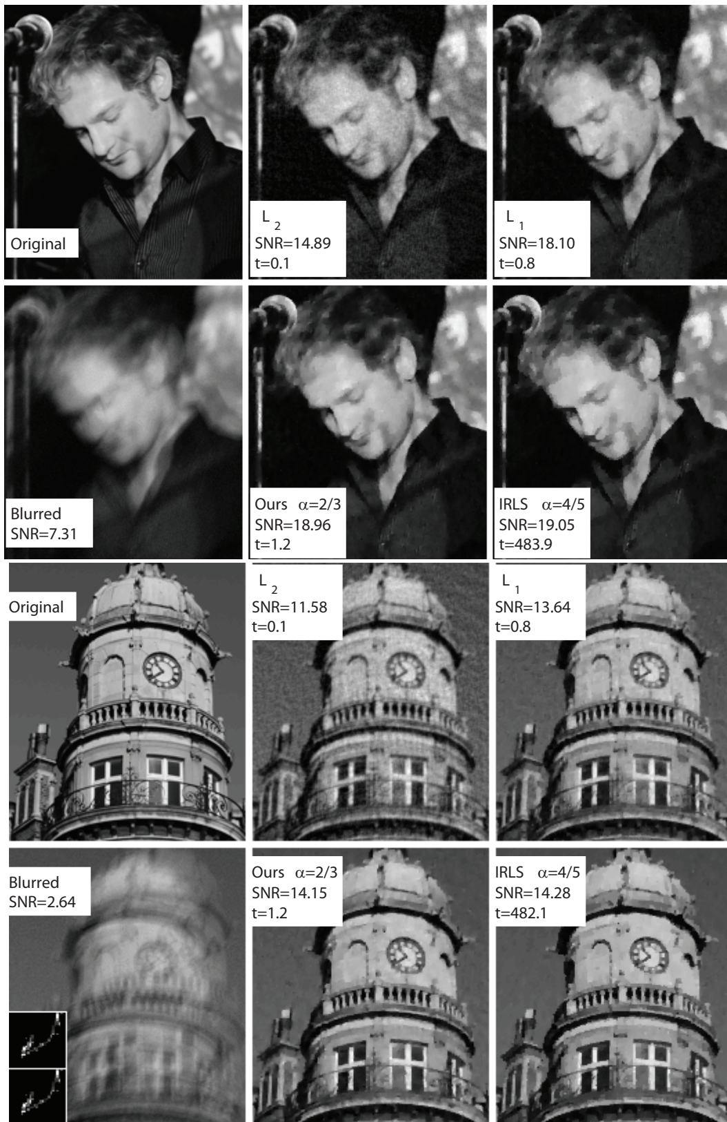
Figure 2: Crops from two images (#1 & #5) being deconvolved by 4 different algorithms, including ours using a 27 \times 27 kernel (#7). In the bottom left inset, we show the original kernel from [12] (lower) and the perturbed version provided to the algorithms (upper), to make the problem more realistic. This figure is best viewed on screen, rather than in print.
