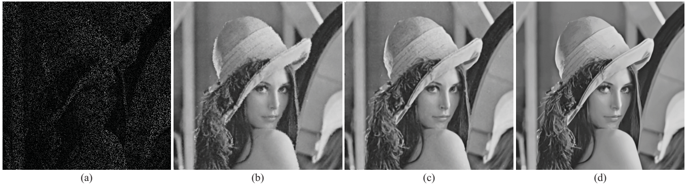
Fig. 9. Image reconstruction performance comparison from irregular samples for Lena image. (a) Irregularly sampled data set (15% of pixels at random locations are preserved). (b) Delaunay-spline interpolation (PSNR = 28.86 dB, SSIM = 0.8419). (c) Iterative steering kernel regression [46] (PSNR = 29.80 dB, SSIM = 0.8524). (d) SAIST (PSNR = 31.32 dB, SSIM = 0.8861).
